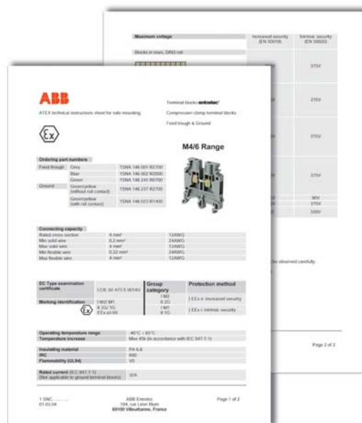
example of terminal blocks technical instruction sheet
